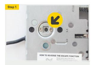
Select escape side (internal facing of door). Screws must be fitted on internal side of mortice lock.
