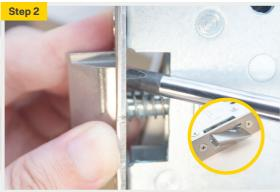
Hand the latch (optional). Push from the inside and twist to change direction (leverage tool required).
